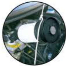
brake bleeding operation.
