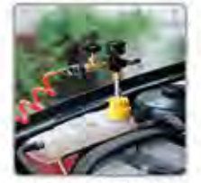
Pressure testing by hand pump
